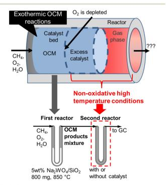
Fig. 1 Schematic representation of the two-stage reactor that mimics industrial reactors.
