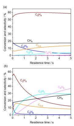
Fig. 4 Simulated product distribution and CH<sub>4</sub> conversion at (a) 850 and (b) 1000 °C using KAM1-GS gas phase kinetics. Inlet gas composition was given by the experimentally obtained values from the outlet of the first reactor. The corresponding mole fractions are shown in Fig. S3.†
