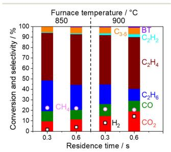
Fig. 2 Product distribution and CH<sub>4</sub> conversion measured with a single quartz tube reactor using 800 mg of 5 wt% Na<sub>2</sub>WO<sub>4</sub>/SiO<sub>2</sub> under  $\rm O_2$  depletion conditions (850 or 900 °C, CH<sub>4</sub> 10 kPa, O<sub>2</sub> 1.7 kPa, H<sub>2</sub>O 1.7 kPa, total pressure 101 kPa, Ar balance, 40 or 80 mL min<sup>-1</sup>). The residence time was calculated by using the volume occupied by the catalysts in the quartz tube. BT denotes benzene and toluene.
