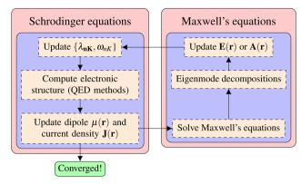
Fig. 8 Self-consistent loop between two sets of equations. The current density from the QED solvers is used to update EM fields. The selfconsistency between Maxwell and Schrödinger equation can be bypassed (in the linear-response regime) by using the pre-calculated Dyadic Green's
