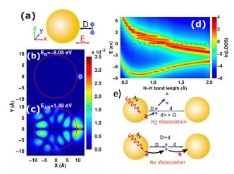
Fig. 4 (a) Schematic diagram of H<sub>2</sub> molecule adsorbed on the NP surface. (b) and (c) Spatial distribution of the bonding and antibonding orbitals of H2 on Jellium NP. (d) Local DOS of bonding and antibonding orbitals of H2 modules as a function of H-H bond length. (e) Depending on the symmetry, the H<sub>2</sub> dissociation can be suppressed or restored in the plasmonic dimer. Figures are adapted with permission from ref. 109. Copyright 2018 American Chemical Society.
