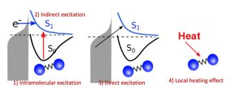
Fig. 3 Proposed mechanisms of plasmon-mediated reactivities. (1) Enhanced intramolecular excitation, (2) indirect charge transfer, (3) direct charge transfer, and (4) local heating
