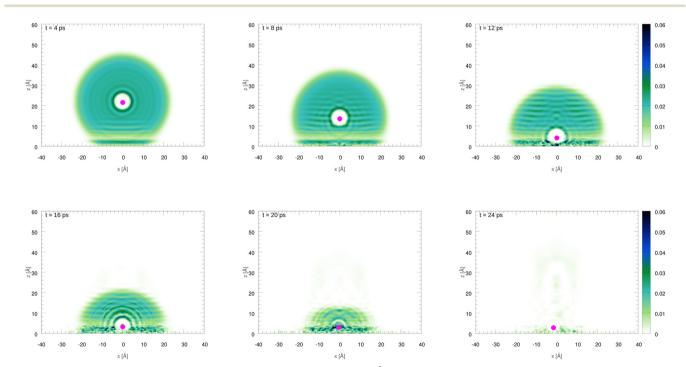
Fig. 3 Two-dimensional (2D) snapshots showing the time evolution of the  $Aga^4$ He<sub>1000</sub> droplet at impact with the graphene surface. The z axis is oriented along the surface normal direction
