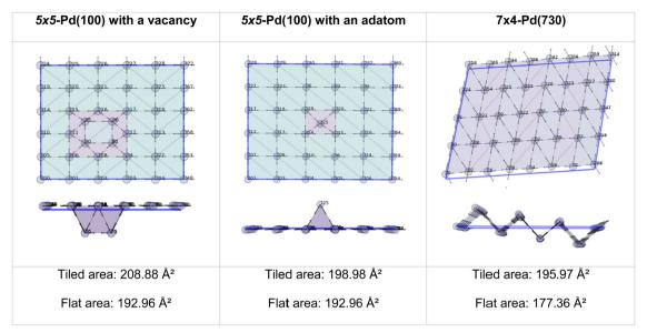
Fig. 4 Top and side view of 3 Pd-surface representations with a vacancy (left), an adatom (middle), and a step (right).
