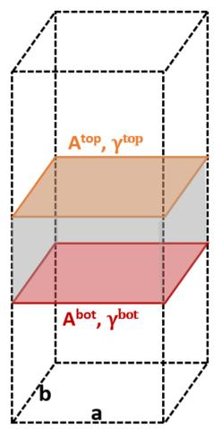
Fig. 1 Illustration of the metal slabs; a and b indicate the periodic cell lattice of the x- and y-axis, and A and  $\gamma$  are the area and surface energies of the top and bottom sides of the slab
