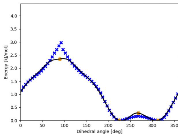
Fig. 5 Dense DFT scan (blue xs) for the intermolecular torsion within the  $\pi$ -bonded methanol–furan complex with CC energies for the optimized stationary points (orange circles). The optimized fit (black line) using eqn (3) maintains the shape from the DFT points while monotonously and differentially touching the stationary points.
