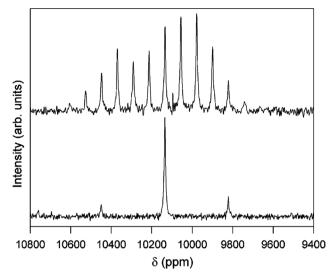
Fig. 12  $^{1}\text{H}-^{103}\text{Rh}$  CP-MAS NMR spectra of  $[[(\text{H}_{2}\text{O})_{4}\text{Rh}(\mu_{2}-\text{OH})_{2}\text{Rh}-$ (H<sub>2</sub>O)<sub>4</sub>],(dmtos)<sub>4</sub>]·8H<sub>2</sub>O comparing spinning rates of 1.0 (top) and 4.0 kHz (bottom). Both spectra acquired with 8 ms contact time, 5 s relaxation delay for 12 000 (top) and 15 800 (bottom) acquisitions.<sup>37</sup> Reproduced from the ref. 37 with permission from the American Chemical Society, copyright 2006.
