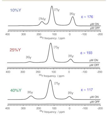
Fig. 3 <sup>89</sup>Y MAS NMR Hahn-echo spectra from co-precipitated ceria samples with various levels (10, 25 and 40%) of  $Y_2O_3$  substitution and 0.1% Gd<sub>2</sub>O<sub>3</sub> showing the signal enhancement (ɛ) via DNP when microwaves (μW) are applied, with the different yttrium coordinations [x]Y observed.<sup>53</sup> Reproduced from ref. 53 with permission from the American Chemical Society, copyright 2021.
