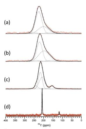
Fig. 9 <sup>89</sup>Y CPMG MAS NMR spectra of  $Y_xSc_{2-x}Si_2O_7$  with (a) x = 0.5, (b) 1.0, (c) 1.5 and (d) 2.0. As scandium is added the appearance of more lines suggests inequivalent sites result from differing NNN yttrium and scandium. 100 Reproduced from ref. 100 with permission from the International Union of Crystallography, copyright 2011.
