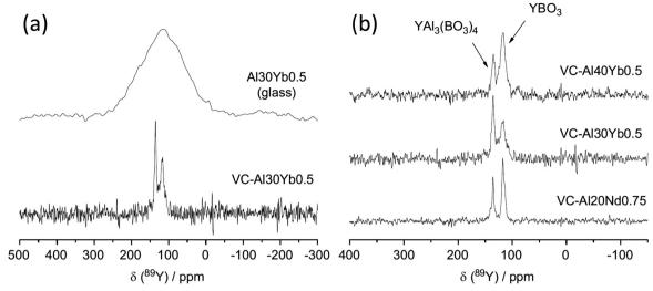
Fig. 10 Application of <sup>89</sup>Y MAS NMR to probe glass to ceramic transitions, with an example given for (a) (Y<sub>2</sub>O<sub>3</sub>)<sub>0.1</sub>(Al<sub>2</sub>O<sub>3</sub>)<sub>0.3</sub>(B<sub>2</sub>O<sub>3</sub>)<sub>0.6</sub> (Al30) Yb-doped sample and (b) comparison of the major yttrium phases that form for different aluminium levels as well as a comparison of ytterbium to neodymium. 105 Reproduced from ref. 105 with permission from Elsevier, copyright 2012.
