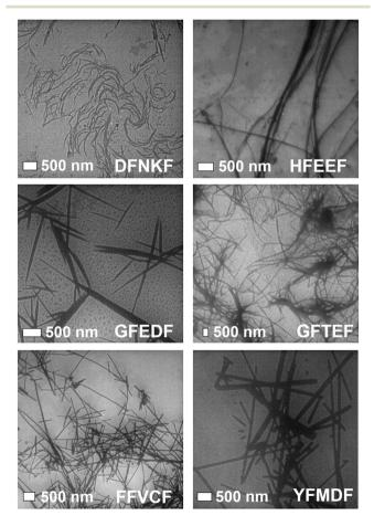
Fig. 5 TEM images of the supramolecular structures formed in water (0.4 mM, aging 48 h) by some of the pentapeptides studied in this work.
