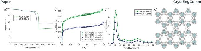
Fig. 4 a) Thermogravimetric analyses of GUF-12(Zr) and GUF-12(Hf) in air. b)  $N_2$  adsorption desorption isotherms (77 K) of GUF-12(Zr) and GUF-12(Hf) with c) pore-size distributions ( $N_2$  at 77 K on carbon, slit pore, QSDFT, equilibrium model) calculated from the isotherms. d) Portion of the DFT model structure of GUF-12(Zr) viewed down the crystallographic c axis to visualise the hexagonal channel 11 Å in diameter.
