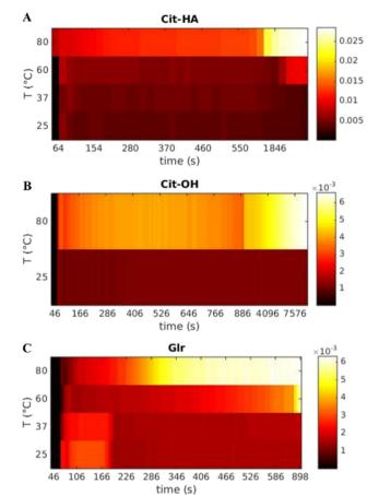
Fig. 3 Bivariate mesh of the integrated SAXS intensity as a function of time and temperature for each carboxylate molecule used. (A) Cit, (B) CitOH, and (C) Glr.
