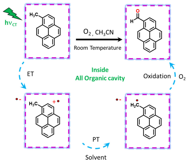
Fig. 4 Photoreaction scheme of CT-mediated C–H functionalization inside ExBox 4+ . CT excitation leads to ET, after which the PT step generates neutral radicals on the benzylic carbons, which undergo oxidation.
