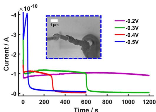
Fig. 3  $i$  vs.  $t$  plots recorded during the potentiostatic ( $E_{\text{app}} = -0.20$  –  $-0.50$ ) V single-barrel SECCM eATRP/FRP of Am using  $[\text{Am}]:[\text{HEBiB}]:[\text{Cu}^{\text{II}}]:[\text{TPMA}] = [20]:[1]:[0.5]:[0.625]$ ; (inset) SEM image of a gel-like feature formed when  $E_{\text{app}} = -0.50$  V.
