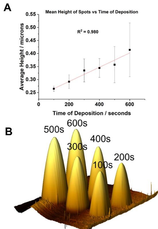
Fig. 4 Si-eATRP of Am at a SAM-functionalised gold electrode using  $[\text{Am}] = 10$  wt% and  $[\text{Cu}^{\text{II}}/\text{TPMA}] = 6.9$  mM; (A) feature height as function of reaction time; (B) 3D representation of the AFM image of features deposited at  $E_{\text{app}} = -0.15$  V at increasing reaction times (100–600 s).
