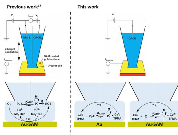
**Fig. 1** Schematic showing the operationally complex dual-barrel SECCM configuration and  $\text{Cu}/\text{Me}_6\text{Tren}$  as a catalyst for localised eATRP which was found to proceed with a competing undesirable ROS-initiated mechanism (left).<sup>17</sup> Here we employ simplified single-barrel SECCM for the first time to control eATRP both at and from the surface of a gold electrode (right).
