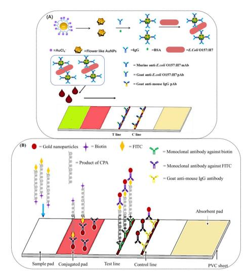
Fig. 7 (A) Surface functionalization of tipped flower-like AuNPs with antibody I (murine anti-E. coli O157:H7 mAb) and BSA; schematic illustration of the immunochromatographic detection of E. coli O157:H7. Figure adapted from Zhang et al., Langmuir, 2015, 31, 5537-5544. (B) Schematic diagram of the cross-priming amplification (CPA)-strip assay. Figure adapted from Gao et al., Sens. Actuators B Chem., 2018, 274, 304-309.
