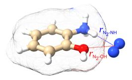
Fig. 2 The two variations of calculating interaction potentials with N<sub>2</sub> depicted for N-protonated 2-aminophenol. In the averaged N2 version, the potential is calculated from each atom of the ion to both atoms of N<sub>2</sub>, and subsequently averaged. In the centre of mass version, the potential is calculated from each atom of the ion to the centre of mass of the N2. Isosurfaces correspond to the envelope of vdW radii of the atoms contained within the molecule.
