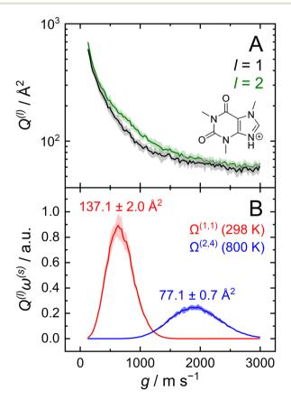
Fig. 4 (A) Momentum transfer integrals and (B) CCS integrands of protonated caffeine. The standard deviations from eqn (12b) are shown as shaded areas, and the final uncertainty for  $\Omega^{(l,s)}$  corresponds to that from eqn (13). CCS calculations were performed using itn = 10, inp = 104, imp= 512 and T = 298 K (panel B; red) for  $\Omega^{(1,1)}$ , and  $T_{\rm eff,max}$  = 800 K for  $\Omega^{(2,4)}$  (panel B; blue).
