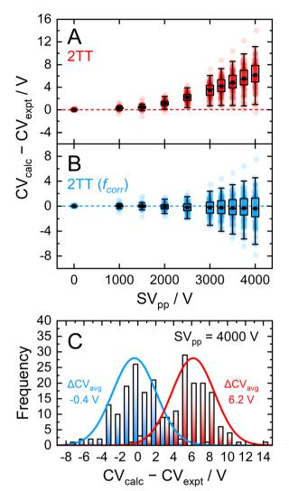
**Fig. 7** Comparison of measured vs. calculated dispersion plots over a range of separation field amplitudes as box plots for (A) uncorrected 2TT and (B) 2TT including the empirical correction employing  $A_{\rm avg}$  and  $B_{\rm avg}$ . Panel (C) shows the distribution of CV deviations using the uncorrected and empirically correct 2TT at the highest SV<sub>pp</sub> (4000 V).
