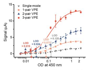
Fig. 3 Redox cycling of TMB using the vertically paired electrode (VPE). (a) Redox cycling of TMB using the alternating potential of the collector electrode. (b) Standard curve for the redox cycling of ox-TMB-2 at different pairs of electrodes. (c) Comparison of the simulation and experimental data of the redox cycling signal for different electrode gaps. (d) Comparison of the simulated and experimental data of the redox cycling signal for different electrode pairs.
