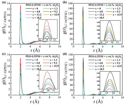
Fig. 5 RDFs of (a) Li<sup>+</sup>-O(PEO) at 333 K, (b) Li<sup>+</sup>-O(TFSI) at 333 K, (c) Li<sup>+</sup>-O(PEO) at 300 K, and (d) Li<sup>+</sup>-O(TFSI) at 300 K in the SC systems. PEO-LiTFSI + x wt%  $Al_2O_3$  represents PEO-LiTFSI with x wt%  $Al_2O_3$ . x is the mass fraction of  $Al_2O_3$ . The insets show an enlargement of the first coordination shell.
