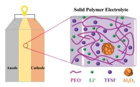
Structures of the solid-state battery and SPE filled with Al<sub>2</sub>O<sub>3</sub>.
