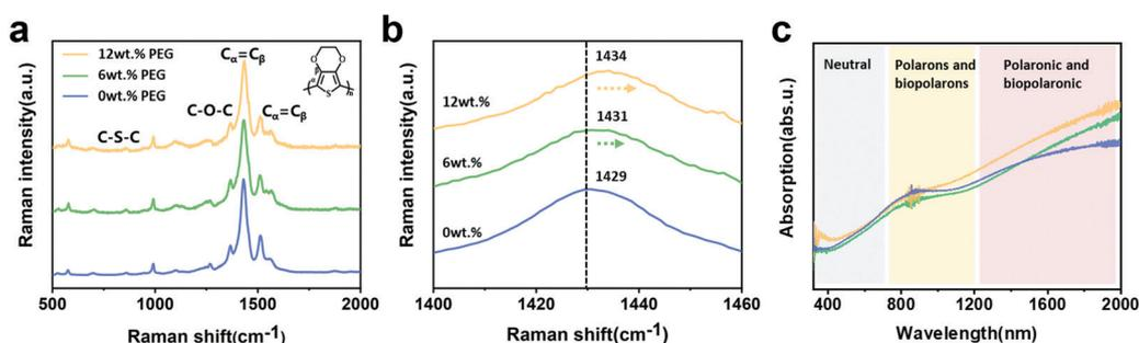
Fig. 2 The microstructure analysis of the VPP PEDOT film fabricated *via* vapor phase polymerization. (a–c) Raman and UV-Vis-NIR spectra of PEDOT film with 0, 6, 12 wt% PEG additions, where (b) is an enlarged image of the Raman spectra near the symmetric  $C_\alpha = C_\beta$  ( $-\text{O}$ ) stretch absorption band.
