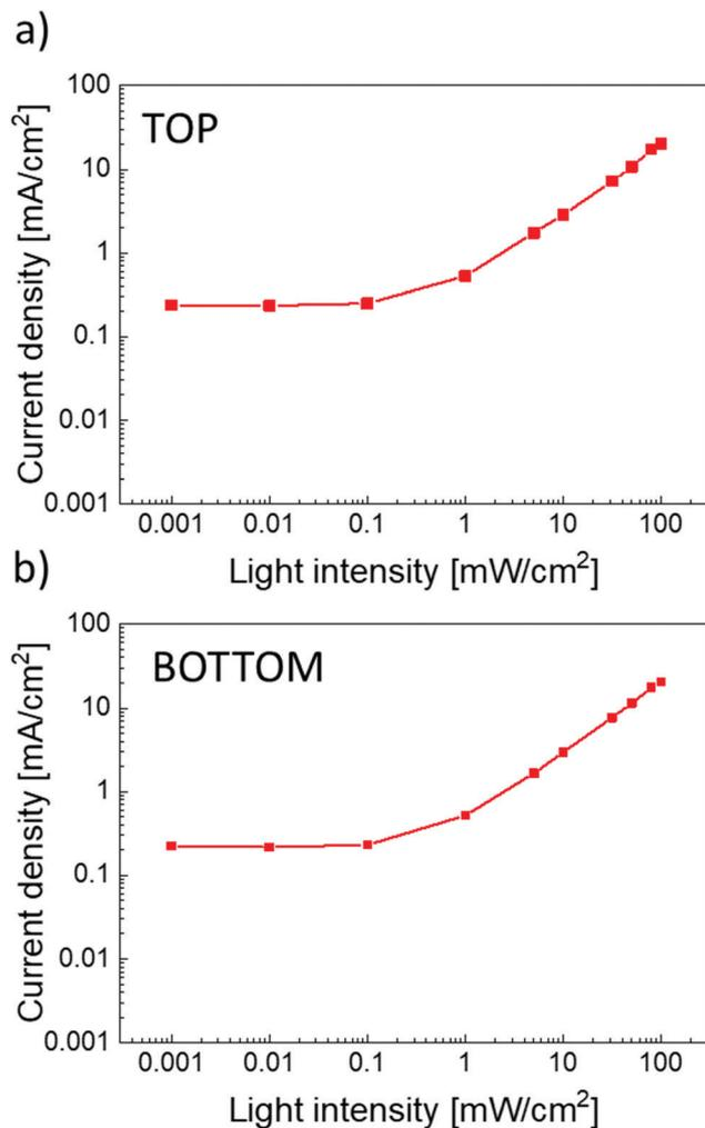
Fig. 4 Linearity (current density vs. light power) of the semitransparent (ITO top contact)  $\text{MA}_{0.3}\text{FA}_{0.7}\text{Pb}_{0.5}\text{Sn}_{0.5}\text{I}_3$  perovskite photodetector illuminated from the (a) top and (b) bottom.
