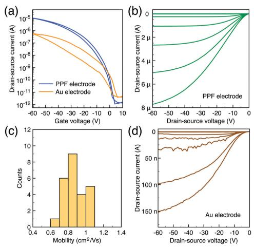
Fig. 4 (a) Transfer I-V curve of DNTT transistors based on PPF and Au electrodes. (b) Output I-V curve of DNTT transistors based on PPF electrodes; the  $V_{\rm G}$  voltage step is 10 V. (c) Mobility histogram of 25 devices. (d) Output I-V curve of DNTT transistors based on Au electrodes; the  $V_{\rm G}$  voltage step is 10 V.
