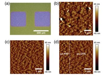
**Fig. 3** (a) Optical image of bottom contact DNTT OFETs. (b) AFM morphology of DNTT deposited on the PPF electrode surface. (c) AFM morphology of DNTT deposited on the OTS modified SAM. (d) AFM morphology of DNTT deposition at the boundary between the electrode and dielectric layer.
