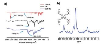
Fig. 1 (a) FT-IR spectra of TPE-Al, TPC and COP-Ta. (b) Solid-state <sup>13</sup>C CP-MAS NMR of COP-Ta.
