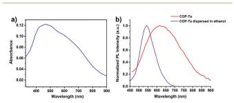
Fig. 2 (a) The UV absorption spectrum of COP-Ta in the solid state. (b) Fluorescence spectra of COP-Ta in the solid state (red) and dispersed in ethanol (purple), respectively ( $\lambda_{ex}$  = 365 nm).
