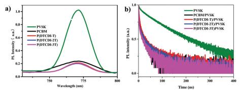
Fig. 4 (a) Steady-state photoluminescence (PL) spectra, and (b) time-resolved photoluminescence (TRPL) decay traces of the perovskite films (PVSK) and ETL-covered perovskite films.
