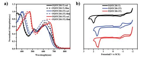
Fig. 1 (a) Optical absorption spectra of P(DTCDI-T), P(DTCDI-2T) and P(DTCDI-3T). (b) Cyclic voltammograms of P(DTCDI-T), P(DTCDI-2T) and P(DTCDI-3T) thin films measured in 0.1 M  $\rm Bu_4N^+PF_6^-$  acetonitrile solution with a scan rate of 100 mV s<sup>-1</sup>.
