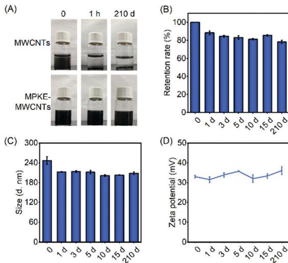
**Fig. 3** Dispersion stability of MPKE-MWCNTs. (A) Images of MWCNTs or MPKE-MWCNTs dispersed in water for different periods. (B) The normalized retention rate of MPKE-MWCNTs dispersed in water for different periods. (C) Particle size and (D) zeta potential of MPKE-MWCNTs dispersed in water for different periods. (h: hour and d: day).
