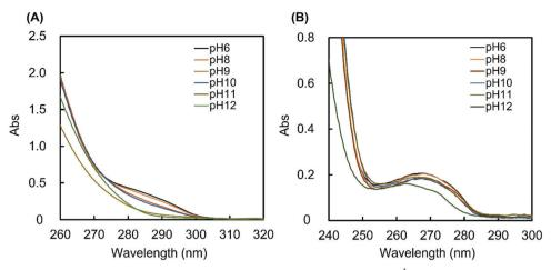
Fig. 2 The UV spectra of (A) PMB-MAPBA and (B) PMB-VPBA solution. The UV spectra of 1 mg mL<sup>-1</sup> polymer solutions were measured at 25 °C using buffers with pH values of 6-12.
