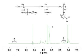
Fig. 1 The <sup>1</sup>H-NMR spectrum of PMB-MAPBA in C<sub>2</sub>D<sub>5</sub>OD.
