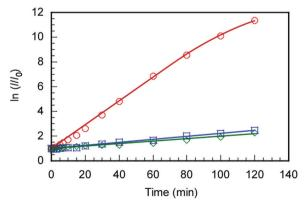
Fig. 7 Changes in SOSG fluorescence intensity (2  $\mu$ M) with C<sub>70</sub>/EUM at  $[C_{70}]_s = 0.03 \text{ g L}^{-1}$  ( $\bigcirc$ ), without  $C_{70}$  ( $\bigcirc$ ), and without EUM and  $C_{70}$  ( $\bigcirc$ ) as a function of irradiation time at 25  $^{\circ}$ C; I and I $_{0}$  were the fluorescence intensities at the maximum wavelength (525 nm) after and before 590 nm light irradiation.
