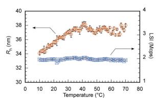
Fig. 6 Hydrodynamic radius ( $R_h$ ,  $\bigcirc$ ) and light scattering intensity (LSI,  $\bigcirc$ ) of  $C_{70}/EUM$  at  $C_p = 2 \text{ g L}^{-1}$  and  $[C_{70}]_s = 0.313 \text{ g L}^{-1}$  in PBS as a function of temperature
