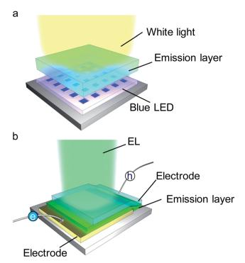
Fig. 7 Cartoon illustrations of (a) a down-conversion LED and (b) a direct-conversion LED.
