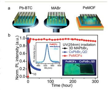
Fig. 9 (a) Illustration of the PeMOF thin film fabrication process via a two-step spin coating method. (b) Time evolution of the normalized photoluminescence intensities of the 3D MAPbBr<sub>3</sub> thin film, CsPbBr<sub>3</sub> QD thin film and PeMOF thin film. The PL spectrum for a PeMOF thin film before and after UV irradiation is plotted in the inset, and a photo of the PeMOF versus QD thin films after aging is shown in the same plot. Reproduced from ref. 20 with permission.
