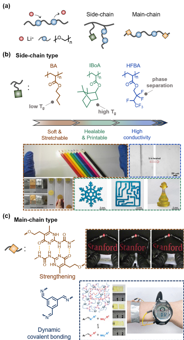
Fig. 10 \text{Li}^+ -Based liquid-free SICs. (a) Schematics of conduction mechanism and types of \text{Li}^+ -based liquid-free SICs. (b) Examples of side-chain-type liquid-free SICs. Engineering co-monomers endows diverse properties to liquid-free SICs. Reproduced with permission from ref. 55. Copyright 2018, Springer Nature. Reproduced with permission from ref. 111 and 116. Copyright 2021, Wiley-VCH. (c) Examples of main-chain-type liquid-free SICs. Reproduced with permission from ref. 32. Copyright 2019, Springer Nature. Reproduced with permission from ref. 112. Copyright 2021, The American Chemical Society.
