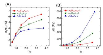
Fig. 5 (A) Ratio of Chebyshev elastic coefficients  $(e_3/e_1)$ , and (B) energy dissipated ( $\Delta E$ ) over a strain cycle for  $A_{25}B_{104}A_{25}-L$ ,  $A_{12}B_{96}A_{12}-L$ , and  $A_8B_{54}A_8$ -L as a function of  $\gamma_0 = 0.61-3.50$
