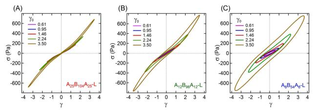
Fig. 3 Lissajous plots obtained from amplitude sweep experiments displaying the shear stress ( $\sigma$ ) vs. intracycle strain ( $\gamma$ ) for (A) A<sub>25</sub>B<sub>104</sub>A<sub>25</sub>-L, (B) A<sub>12</sub>B<sub>96</sub>A<sub>12</sub>-L, and (C) A<sub>8</sub>B<sub>54</sub>A<sub>8</sub>-L for  $\gamma_0 \approx 0.61$ , 0.95, 1.46, 2.24, and 3.50. The experiments were performed using oscillatory frequency ( $\omega$ ) of 1 rad s<sup>-1</sup>.
