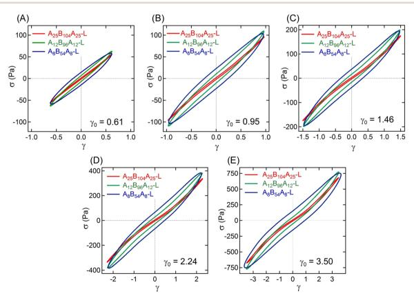
Fig. 4 Lissajous plots for  $A_{25}B_{104}A_{25}$ -L,  $A_{12}B_{96}A_{12}$ -L, and  $A_8B_{54}A_8$ -L obtained from amplitude sweep experiments displaying the shear stress ( $\sigma$ ) vs. intracycle strain ( $\gamma$ ) at  $\gamma_0 \approx$  (A) 0.61, (B) 0.95, (C) 1.46, (D) 2.24, and (E) 3.50. The experiments were performed using  $\omega = 1$  rad s<sup>-1</sup>.
