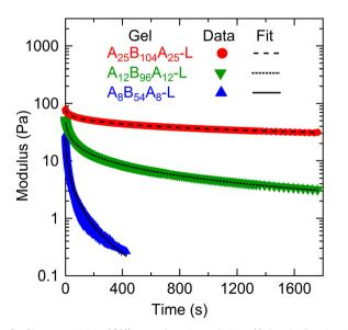
Fig. 6 Shear modulus (G(t)) as a function of time (t) for  $A_{25}B_{104}A_{25}$ -L,  $A_{12}B_{96}A_{12}$ -L, and  $A_8B_{54}A_8$ -L obtained from stress-relaxation experiments for a step-strain of  $\gamma_0$  = 0.01 at  $\approx$  27 °C. The lines represent the fitting of the stretched-exponential model (eqn (3)).
