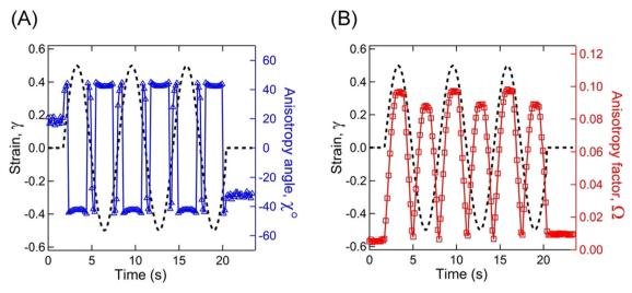
Fig. 11 Estimated anisotropic factor and angle for A<sub>12</sub>B<sub>96</sub>A<sub>12</sub>-H. (A) Strain (γ) on the left-y-axis and anisotropy angle (χ) on the right-y-axis as a function of time. (B)  $\gamma$  on the left-y-axis and anisotropy factor ( $\Omega$ ) on the right-y-axis as a function of time. RheoSAXS experiments were performed with an oscillatory  $\gamma_0 = 0.5 \text{ and } \omega = 1 \text{ rad s}^{-1}$ .
