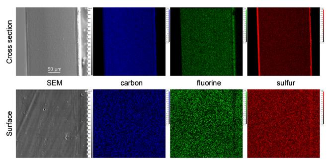
Fig. 4 SEM and EPMA element mapping images (blue: carbon, green: fluorine, and red: sulfur) of cross section and surface of the ionic SMP gel sensor with PEDOT:PSS electrodes on both surfaces of the gel ( $W_{\rm IL}$  = 25 wt%).
