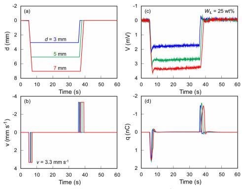
Fig. 7 Relation between input mechanical stimuli of (a) constant bending velocity ( $v = 3.3 \text{ mm s}^{-1}$ ) with (b) different displacements (d = 3, 5, 7 mm) and output electric signals of (c) voltage (V) and (d) electric charge (q) of ionic SMP gel sensor ( $W_{1L} = 25 \text{ wt}$ %).
