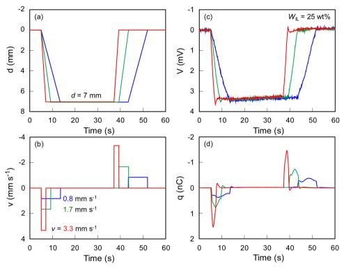
Fig. 6 Relation between input mechanical stimuli of (a) constant bending displacement (d = 7 mm) with (b) different velocities (v = 0.8, 1.7, and 3.3 mm s<sup>-1</sup>) and output electric signals of (c) voltage (V) and (d) electric charge (q) of ionic SMP gel sensor ( $W_{IL} = 25$  wt%).
