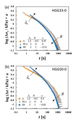
Fig. 5 Failure of the superposition of  $\log \Delta \sigma - \log t$  curves for different types of deformation with various values of  $\lambda_x$  by vertical shift with a factor of a for (a) HGG33-0 and (b) HGG50-0. Qualitative features of the failure of the superposition are common to HGG33-0, HGG50-0 and HGG64-0 (Fig. 4).
