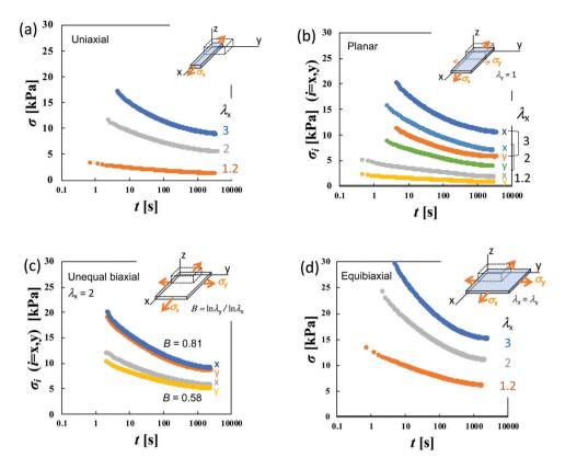
Fig. 3 Elapsed time (t) dependence of nominal stress (σ) for HGG63-0 after the imposition of (a) uniaxial, (b) planar, (c) unequal biaxial and (d) equibiaxial extension with various degrees of imposed stretching
