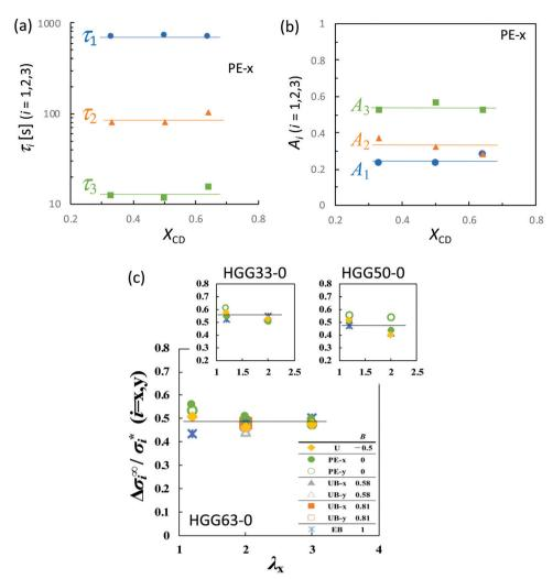
Fig. 7 (a) Relaxation times,  $\tau_i$  (i = 1, 2, and 3) and (b) relaxation strengths,  $A_i$  (i = 1, 2, and 3) as a function of  $X_{CD}$  for  $\sigma_x$  in planar extension. (c) Total stress relaxation ( $\Delta\sigma^{\infty}$ ) in several types of stretching as a function of  $\lambda_x$  for the HG gels with various values of  $X_{CD}$ .  $\Delta\sigma^{\infty}$  is reduced by the initial stress ( $\sigma^*$ ) in each deformation.
