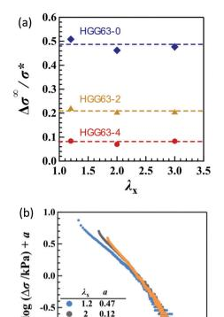
Fig. 8 (a) Total stress relaxation ( $\Delta \sigma^{\infty}$ ) in uniaxial stretching as a function of  $\lambda_x$ for the HG gels with  $X_{CD} = 0.63$  and various concentrations of covalent crosslinks. (b) Failure of the superposition of  $\log \Delta \sigma$  –  $\log t$  curves for uniaxial stretching with various values of  $\lambda_x$  by vertical shift with a factor of a for HGG63-2.
