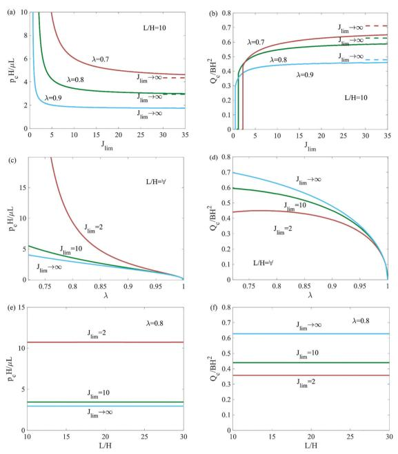
Fig. 5 The critical pressure  $p_c$  and extrusion volume  $Q_c$  for elastic leak as functions of  $J_{lim}$ ,  $\lambda$ , and L/H.
