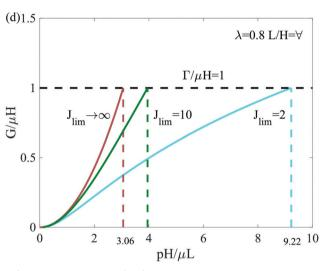
Fig. 6 A model of rupture. (a-c) The model assumes a debonded region of length  $l_c$  located at the bottom of the upstream front of the seal. (d) The relation between energy release rate G and pressure p. A strain-stiffening material will enhance the critical pressure of rupture compared to a neo-Hookean material
