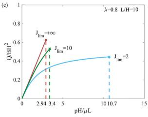
Fig. 4 (a and b) Displacement of seals for both strain-stiffening (open circle) and neo-Hookean (solid line) materials under different fluid pressures. (c) Relation between the fluid pressure p and the extrusion volume Q, plotted in the dimensionless form for both strain-stiffening ( $J_{lim} = 2, 10$ ) and neo-Hookean ( $J_{\text{lim}} \rightarrow \infty$ ) materials. Cross markers are critical points for seals to leak by elastic deformation.
