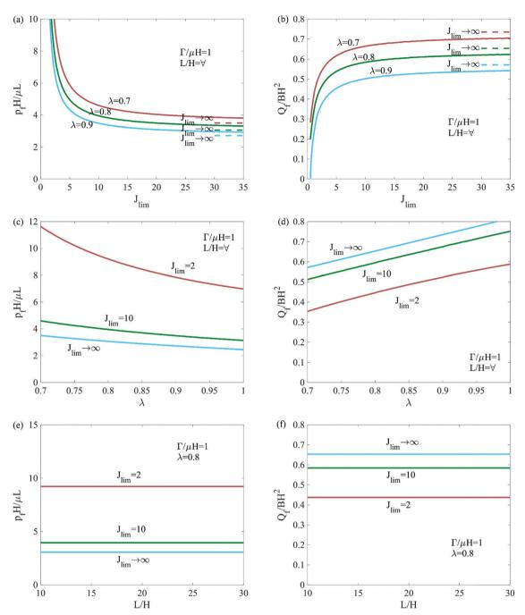
Fig. 7 The pressure  $p_f$  and extrusion volume  $Q_f$  for rupture as functions of  $J_{lim}$ ,  $\lambda$ , and L/H.
