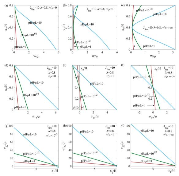
Distributions of the elastic energy density of seal  $W/\mu$  and stresses  $\sigma_{12}$  and  $\sigma_{22}$  under the deformation
