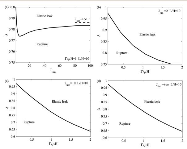
Fig. 8 Leak by elastic deformation and leak by rupture are demarcated on planes of various axes. (a) The diagram in the  $J_{lim}$ - $\lambda$  plane for strain-stiffening seals with the fixed  $\Gamma/\mu H$  and L/H. (b) The diagrams in the  $\Gamma/\mu H - \lambda$  plane for strain-stiffening seals with the fixed  $J_{lim}$  and L/H. (c) The diagrams in the  $\Gamma/\mu H - \lambda$  $\mu H - \lambda$  plane for neo-Hookean seals with the fixed L/H.
