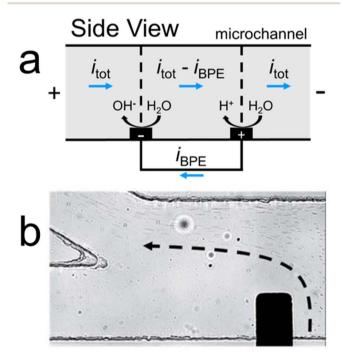
Fig. 4 (a) Schematic illustration of ionic current variations caused by BPEs. Adapted with permission from ChemElectroChem, 2022, 9, e202200251 (Copyright © 2022 WILEY-VCH Verlag GmbH & Co. KGaA, Weinheim). (b) Optical micrograph of a bifurcated microchannel during an electrochemical microplastic separation experiment in buffer-free solution. Adapted from Chem. Sci., 2021, 12, 13744-13755 (copyright © 2022 Royal Society of Chemistry).
