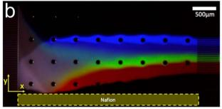
Fig. 2 (a) Schematic illustration of a microfluidic device designed to use ICP for the continuous separation and enrichment of anionic dyes. (b) Fluorescence micrograph of the device shown in (a) when continuously separating and enriching three anionic dyes. Adapted from: *Anal. Chem.*, 2020, **92**, 4866–4874 (copyright © 2011 American Chemical Society).
