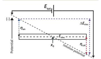
Scheme 2 Schematic representation of the operation of a bipolar electrode. Adapted from: *Angew. Chem., Int. Ed.,* 2013, **52**, 10438–10456 (copyright © 2013 WILEY-VCH Verlag GmbH & Co. KGaA, Weinheim).
