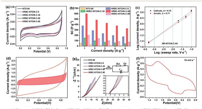
Fig. 5 (a) CV curves of HRBC-NTO/N-C-x and NTO-60 at 0.05 mV s<sup>-1</sup>. (b) The areal capacitance of HRBC-NTO/N-C-x and NTO-60 at various current densities. (c) Linear relationship between log i and log v. (d) Decoupling of the capacitive contributions (red) of HRBC-NTO/N-C-60 at 20 mV S<sup>-1</sup>. (e) The EIS curves of HRBC-NTO/N-C-x and NTO-60. (f) CV curve of the CDI system measured in a 2 mol L<sup>-1</sup> NaCl solution at 10 mV s<sup>-1</sup> via a two-electrode method.
