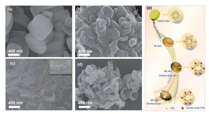
Fig. 2 SEM images of (a)  $NH_2$ -MIL-125, (b) HRBC-MOF-30, (c) HRBC-MOF-60, and (d) HRBC-MOF-90. (e) Schematic illustration of the process of HRBC-MOF-x.
