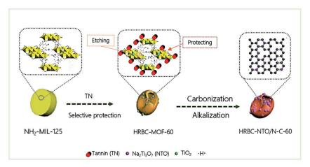
Fig. 1 Schematic illustration of the formation process of HRBC-NTO/N-C-60.
