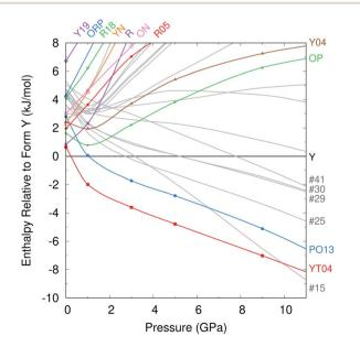
Fig. 4 Enthalpies of the different crystal structures relative to form Y as a function of pressure, in kJ mol<sup>-1</sup>.
