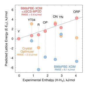
**Fig. 3** Relative lattice energies for seven ROY polymorphs predicted with the CrystalOptimizer potential (orange), B86bPBE-XDM (blue) and B86bPBE-XDM + the SCS-MP2D monomer-correction (red) compared against the experimentally measured relative enthalpies (kJ mol<sup>-1</sup>). Points lying along the solid gray line would represent perfect agreement between the relative theoretical lattice energies and experimental enthalpies.
