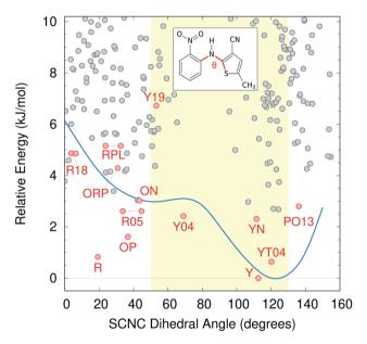
**Fig. 6** ROY crystal structure energy landscape as a function of the intramolecular conformation, as defined by the key SCNC dihedral angle. The gas-phase SCS-MP2D conformational energy scan over this dihedral angle is superimposed on the landscape in blue, while the yellow shaded region indicates the approximate dihedral angle range that leads to yellow polymorphs instead of red/orange ones.
