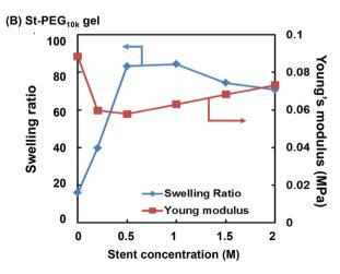
Fig. 4 Effect of stent concentration on the swelling ratios and Young's moduli of the (A) St-PEG<sub>5k</sub> and (B) St-PEG<sub>10k</sub> gels.
