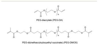
**Fig. 1** Structures of the cross-linkers used in this study: PEG-DA and PEG-DMOS.
