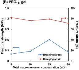
Fig. 3 Effect of total macromonomer concentration (4-arm PEG-SH + PEG-DA) on compressive fracture strength and strain for the (A) PEG<sub>5k</sub> and (B) PEG<sub>10k</sub> gels.
