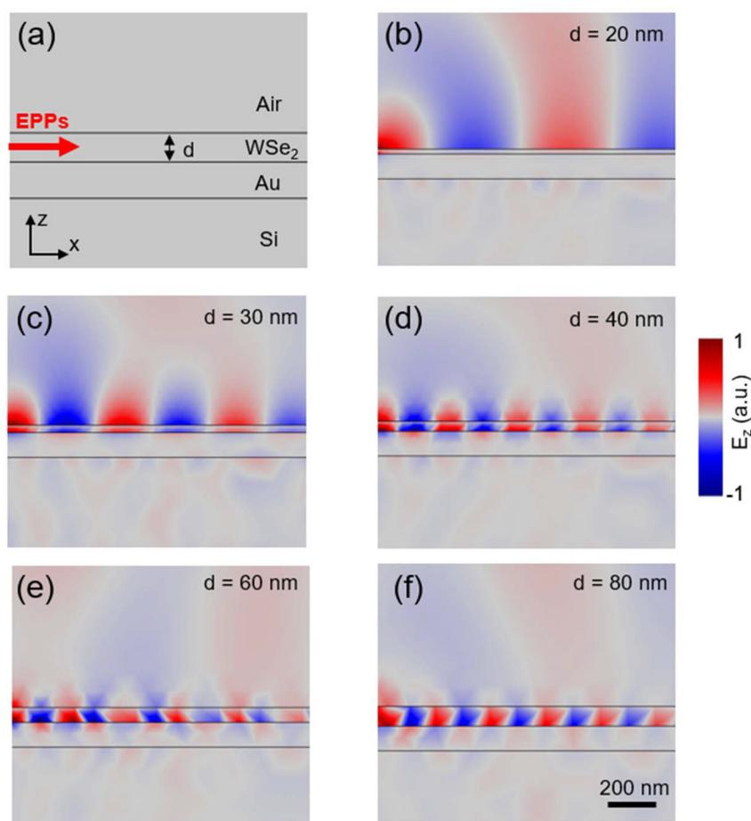
**Fig. 4** (a) Sketch of the air/WSe<sub>2</sub>/Au/SiO<sub>2</sub> four-layer heterostructure model for EPP simulations. (b)–(f) The simulated  $E_z$  field maps of the EPP mode inside the WSe<sub>2</sub>/Au heterostructure with various WSe<sub>2</sub> thicknesses. The excitation energy is  $E = 1.38$  eV.
