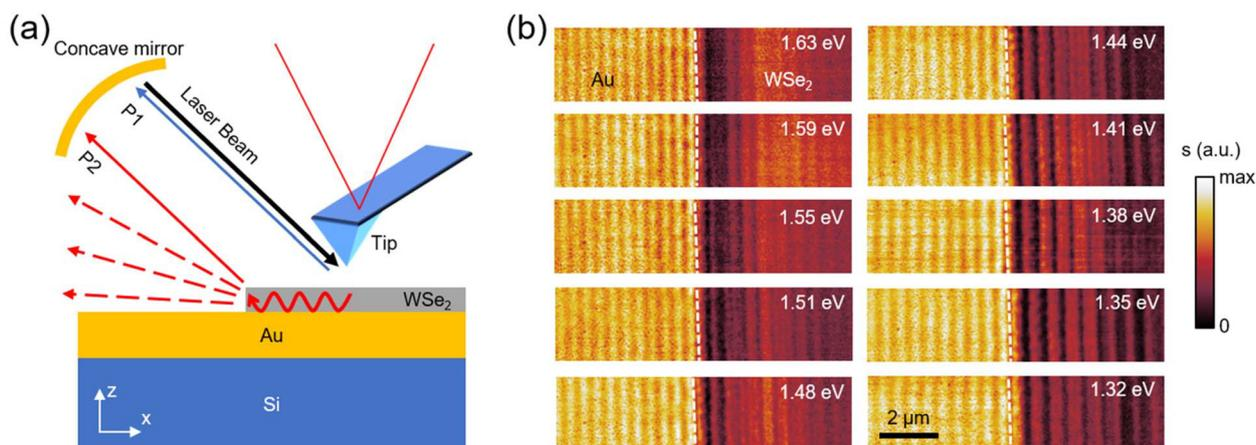
**Fig. 1** (a) Illustration of nano-optical imaging experiment of a WSe<sub>2</sub>/Au heterostructure sample. (b) The near-field amplitude images of a typical WSe<sub>2</sub>/Au heterostructure taken at various excitation energies. The white dashed line marks the edge of the WSe<sub>2</sub> flake.
