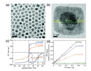
Fig. 9 Stable Fe(0) nanoparticles, designed for optimal MPI performance. (a) Low and (b) high resolution TEM (HRTEM) images of the cubic 14 nm nanoparticles. (c) Hysteresis curves displaying the field-dependent magnetism of 14 and 11 nm Fe(0) nanoparticles. (d) Plot of the MPI signal of the synthesised samples in comparison to that of the reference, VivoTrax, as a function of core mass. Reproduced from ref. 1 with permission from the Royal Society of Chemistry.
