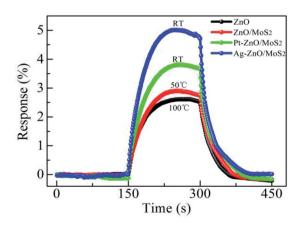
Fig. 10 Sensing responses of pure ZnO, ZnO-MoS<sub>2</sub>, Pt-ZnO-MoS<sub>2</sub> and Ag-ZnO-MoS<sub>2</sub> film sensors towards 100 ppm CO gas (reproduced from ref. 143 with permission from Elsevier).
