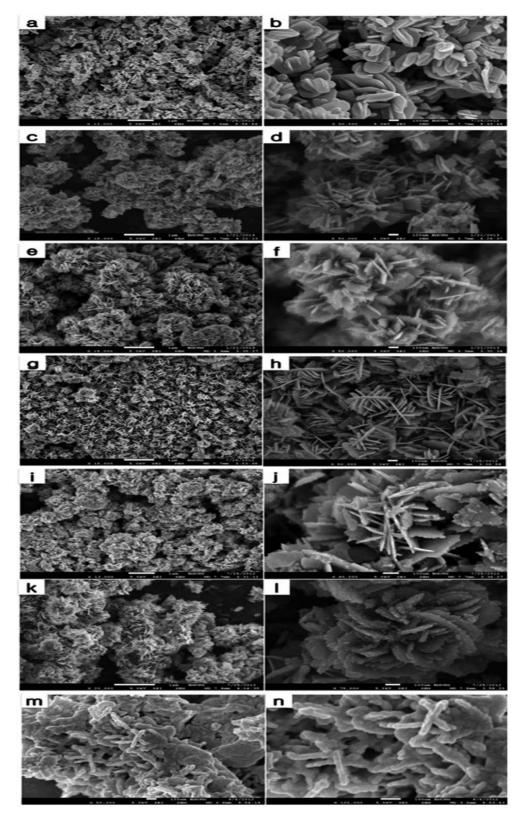
Fig. 2 FESEM images of ZnO prepared using different concentrations of uncooked rice (g): 0 (a and b), 0.25 (c and d), 0.5 (e and f), 1 (g and h), 2 (i and j), 4 (k and l), and 8 (m and n) (reproduced from ref. 84 with permission from Springer).
