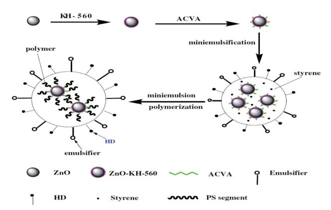
Fig. 5 A schematic diagram showing the synthesis of ZnO/polystyrene nanocomposites by anchoring 4.4'-azobis(4-cyanovaleric acid) (ACVA) onto the surface of ZnO nanoparticles to initiate styrene polymerization (reproduced from ref. 97 with permission from Elsevier).
