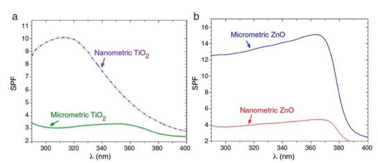
Fig. 16 SPF curves of COLIPA sunscreen incorporating an inorganic UV filter: nanometric (dashed lines) and micrometric (solid lines) (a)  $TiO_2$  and (b) ZnO particles (reproduced from ref. 149 with permission from Elsevier).
