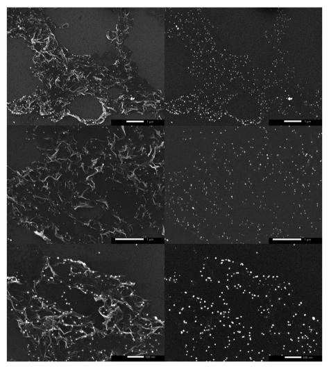
Fig. 5 SEM micrographs of the broken CVD-graphene sheet into smaller structures containing AgNPs owing to sonomechanical treatment in the presence of HNO<sub>3</sub>. Images on the left were taken using the secondary electron detector (SED) whereas those on the right are the representative images taken using the backscattering detector (BED).
