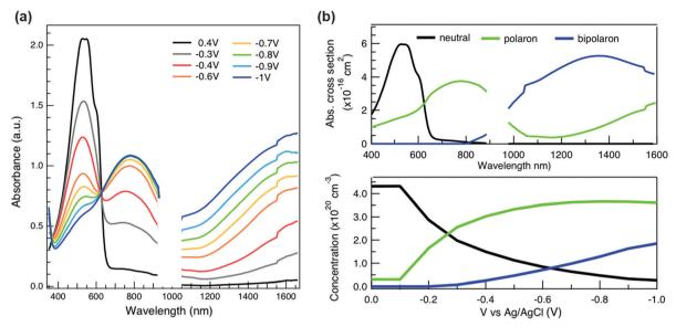
Fig. 3 (a) In situ absorbance spectra of the spin-coated P3HT film at different applied voltages versus Ag/AgCl electrode in 0.1 M KPF<sub>6</sub>/water in steady state conditions. (b) Component spectra (top) and voltage-dependent concentrations (bottom) of the neutral, polaronic and bipolaronic species of electrochemically doped P3HT, as obtained from soft-modeling MCR-ALS analysis of the spectro-electrochemistry spectra
