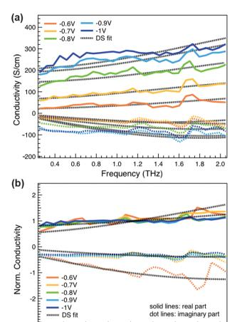
Fig. 2 (a) Complex conductivity spectra of electrochemically doped P3HT at different oxidation potentials versus Ag/AgCl. The real and imaginary parts are shown with solid and dotted lines. (b) Normalized real (solid) and scaled imaginary (dashed) parts of the conductivity at different applied voltages. The fit results from the Drude-Smith model are shown with black dotted lines
