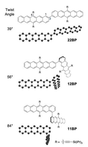
Fig. 1 Minimized geometry revealing increasing interpentacene dihedral (twist) angle going from 22BP (39°), 12BP (56°) to 11BP (84°) (see ESI‡ for details). Only the pentacene monomers and their connectivities are shown in the optimized geometries for clarity. The ethynyl groups are used in determining the optimized geometries since they make a significant difference to the electronic structure. The 1, 2, and 6 positions on the pentacene are labeled on one of the pentacenes in 22BP.
