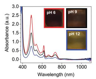
Fig. 4 Reduced absorbance spectra of NDI-F solution at pH 6 (—), 9 (—) and 12 (—). Inset images of the resulting colouration are shown at pH 6, red square, pH 9 black square and pH 12, blue square.
