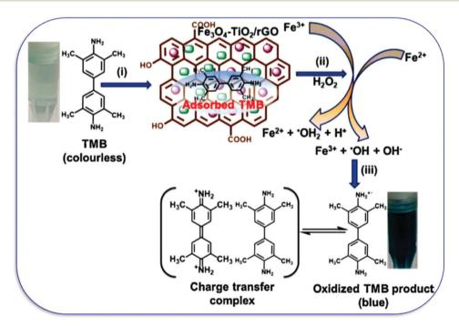
Fig. 12 The peroxidase-like activity of the FTG nanocomposite showing the (i) adsorption of TMB onto the FTG nanocomposite surface, (ii) formation of \*OH by the Fenton reaction, and (iii) TMB oxidation by \*OH radicals. 176 Copyright Elsevier B.V. 2019.
