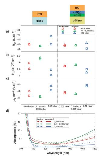
Fig. 2 (a) Sheet resistance  $(R_{sh})$ , (b) free carrier density  $(N_e)$  and (c) electron mobility ( $\mu_e$ ) of PLD ITO films deposited at LP (0.005 mbar); LP with buffer (0.1 + 0.005 mbar) and high pressure (0.02 mbar) on glass (left) and a-Si:H/c-Si stacks (right). (d) Absorptance as a function of wavelength of the ITO films.
