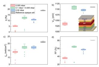
Fig. 3 Statistical distribution of the solar cell parameters for semitransparent perovskite devices with the different PLD ITO deposition pressure conditions. (a) Power conversion efficiency, (b) open-circuit voltage ( $V_{oc}$ ), (c) short-circuit density ( $J_{sc}$ ), and (d) fill factor (FF). Deposition pressure for PLD ITO is indicated in the inset of the graphs. Reference opaque cells with the evaporated Ag rear electrode are shown in grey.
