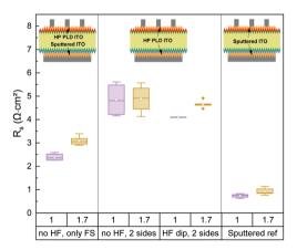
Fig. 6 Comparison of total series resistance ( $R_s$ ) for a set of SHJ cells with PLD ITO at the front and PLD or sputtered rear electrode and Ag grid pitch of 1 and 1.7 mm, respectively. R<sub>s</sub> of the cell with double-sided sputtered ITO is given for reference.
