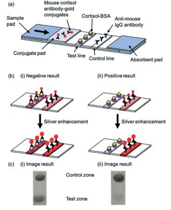
**Fig. 6** Schematic illustration of a competitive salivary cortisol LFA utilising silver enhancement. (a) Schematic of the basic LFA strip and components (b) principle of LFA before and after enhancement for (i) negative result and (ii) positive result (c) image result of the test and control lines for (i) negative result and (ii) positive result. Reproduced with permission. <sup>62</sup> Copyright 2018, PMC.
