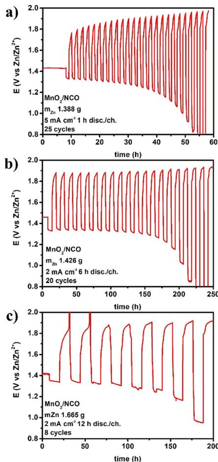
Fig. 4 Electrically rechargeable ZABs (anode paste, GPEs from natural biopolymers, bifunctional cathodes) operated under “long cycles” at (a) 5 mA h cm<sup>-2</sup>, (b) 12 mA h cm<sup>-2</sup>, and (c) 24 mA h cm<sup>-2</sup>.
