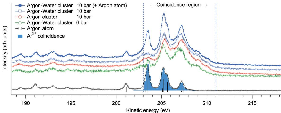
Fig. 1 Overview Auger electron spectra resulting from Ar L-shell ionization measured in non-coincident scanning mode (lines). The  $L_{2,3}M_{2,3}M_{2,3}$  transitions in Ar atoms are also designated (sticks).<sup>15</sup> The same features in clusters, targeted in the electron–ion coincidence measurements, are broader and found at slightly higher kinetic energies.
