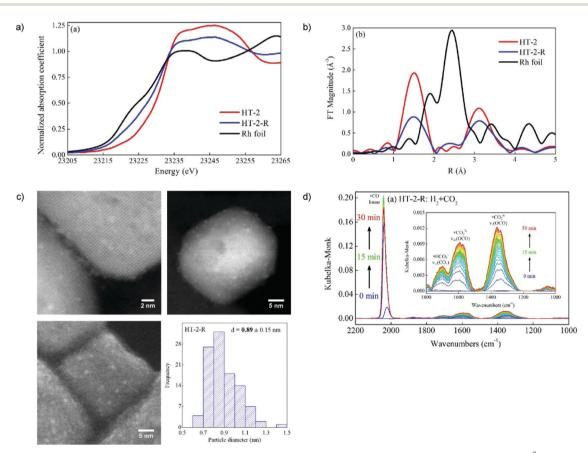
Fig. 2 In situ XAFS data of Rh foil, the HT-2 and HT-2-R samples: (a) XANES region, and (b) Fourier transform magnitudes of the  $k^2$ -weighted EXAFS data. (c) Representative annular dark-field (ADF-)STEM images (top), and high-resolution SEM images (bottom left), and the size distribution of Rh nanoparticles (bottom right) of the HT-2-R sample. (d) In situ DRIFT spectra of CO2 hydrogenation after H2 reduction over HT-2-R. Adapted from ref. 79, Copyright 2018, with permission from Elsevier.
