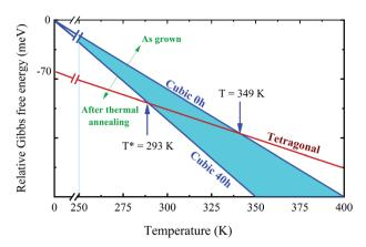
Fig. 8 Schematic of the Gibbs free energy as a function of temperature. At T=0 K, the energies correspond to the internal energy of each system and were computed within the DFT approach and used the cubic system as a reference. As the temperature increases, the configuration entropy is responsible for different phase transition temperatures from tetragonal to cubic, indicated by 293 and 349 K. The configurational entropy is larger for the sample that was annealed for 40 h
