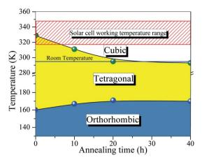
Fig. 6 Phase diagram proposed for the  $MAPbl_3$  halide perovskite taking into account the observed shift in the phase transition temperature with different annealing conditions. The horizontal bar corresponds to room temperature, and the hachured region indicates the solar cell working temperature range.
