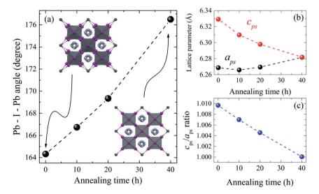
Fig. 5 Structural parameters of the MAPbI<sub>3</sub> samples submitted to thermal annealing at 250 °C (523 K) and different annealing time. (a) The Pb-I-Pb bond angle changing to almost  $180^{\circ}$ ; insets illustrate rotation of PbI<sub>6</sub> octahedra along the c-axis. (b) Pseudocubic lattice parameters and (c) variation of lattice parameter ratio,  $c_{\rm ps}/a_{\rm ps}$ , which reaches 1 for 40 h annealing time.
