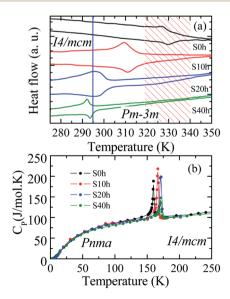
Fig. 3 (a) DSC cycling measurements. The vertical bar indicates the room temperature and the hachured region of the solar cell working temperature range. (b) Molar heat capacity as a function of temperature of pelletized MAPbI $_3$  annealed at  $T_A=250~^{\circ}\text{C}$  (523 K) for different annealing times.
