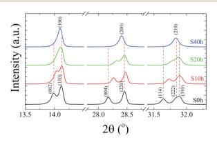
Fig. 2 Room-temperature X-ray diffraction patterns of the pelletized MAPbl<sub>3</sub> sample after being submitted to a heat treatment at T = 250 °C for different annealing times, t = 0, 10, 20, and 40 h.
