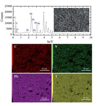
Fig. 1 EDS spectrum and elemental map analysis obtained from a fractured surface of S40 h sample.
