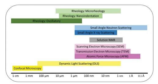
Fig. 5 Characterization techniques used to measure self-assembly and gel properties and their functional length scales.
