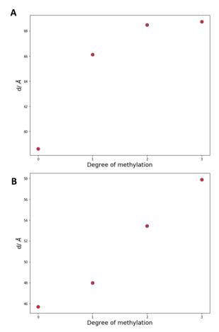
Fig. 8 Effect of headgroup methylation on d spacings in 2:1 palmitic acid: phospholipid mixtures. (A) d spacing values of the L<sub> $\beta$ </sub> phase at 50 °C. (B) d spacing values of the  $H_{II}$  phase at 65 °C. The error bars are approximately the size of the plotted data points.
