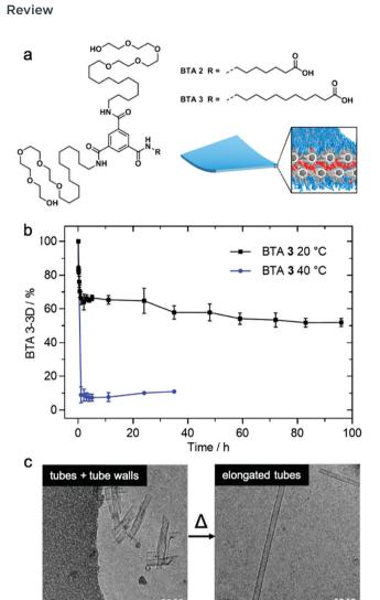
Fig. 7 (a) Chemical structure of BTA 2 and BTA 3, which are schematically illustrated to form a membrane packing morphology. (b) Exchange rates illustrated by HDX-MS reveals the conversion of BTA 3-3D into BTA 3-6D at 20 and 40 °C. (c) Cryo-TEM images of BTA 3 show a transformation from short nanotubes with ill-formed tube walls to well-formed nanotubes after heating from 20 °C to 60 °C. Adapted from ref. 111, Copyright 2018 American Chemical Society
